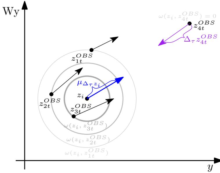
Figure 4: Local mean estimation of the *expected movement* from  $z_i$  ( $\hat{\mu}_{\Delta_\tau z_i}$ ) from four observed movement vectors ( $z_{jt}^{OBS}$ ). Probabilities attached to each observed movement vectors, given by  $\omega(z_i, z_{jt}^{OBS})$ , are a negative function of the distance between  $z_i$  and  $z_{jt}^{OBS}$ .
